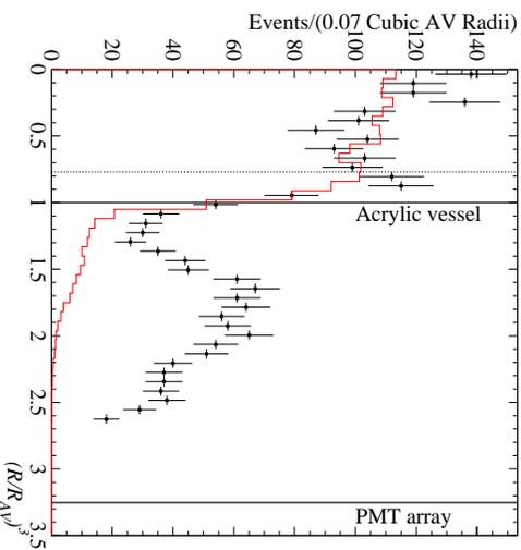
FIG. 1. Distribution of event candidates with  $T_{\text{eff}} \geq 6.75$  MeV as a function of the volume weighted radial variable  $(R/R_{\text{AV}})^3$ . The Monte Carlo simulation of the signals, weighted by the results from the signal extraction, is shown as a histogram. The dotted line indicates the fiducial volume cut used in this analysis.
