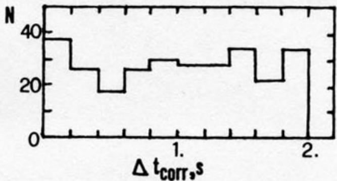
The distribution of time differences between the pulses in the pairs ( $\Delta t = 2 \text{ s}$ ) for the whole data set excluding the interval of interest
