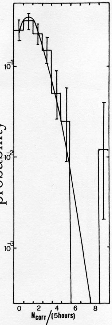
The probability distribution of the counting rate of pairs of correlated pulses per 5 hours and the poissonian fit to this distribution;  $\langle n_{\text{corr}} \rangle = 1.46 / (5 \text{ hours})$ ,  $\Delta T = 2 \text{ s}$
