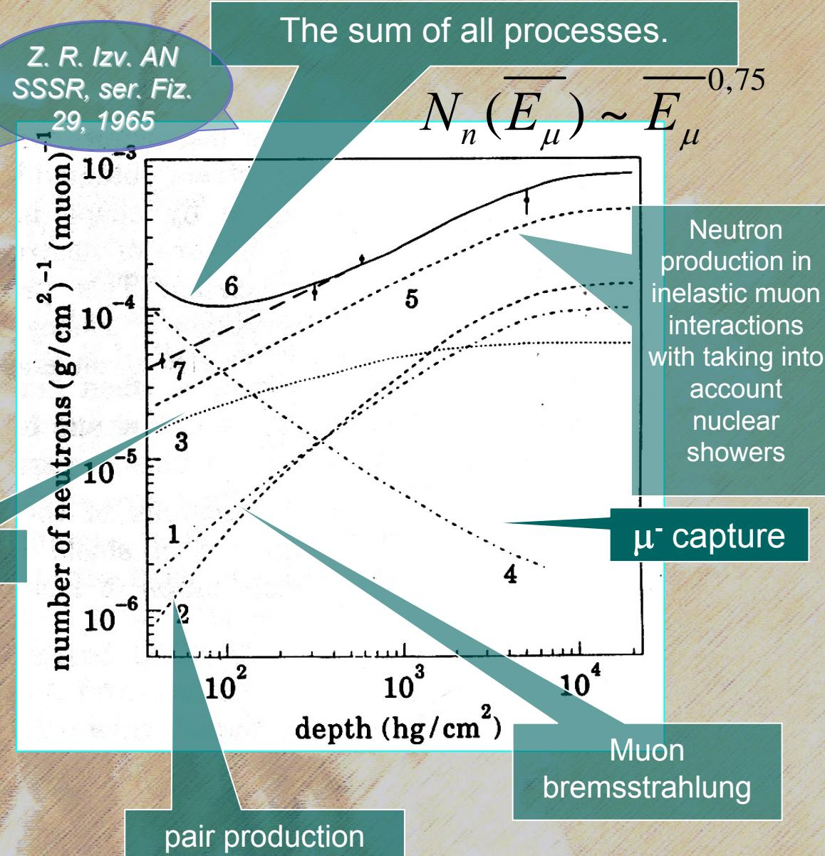
The number of generated neutrons per 1 muon per 1 g/cm<sup>2</sup> vs the depth from the top of the atmosphere.
