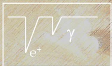
$$n + H \rightarrow d + \gamma \quad (E_\gamma = 2.2\text{MeV}) \\ n + {}^{56}Fe \rightarrow {}^{57}Fe + \sum \gamma \quad (E_\gamma = 10.16\text{MeV}) \quad \left. \right\} \tau \approx 185\mu s$$
