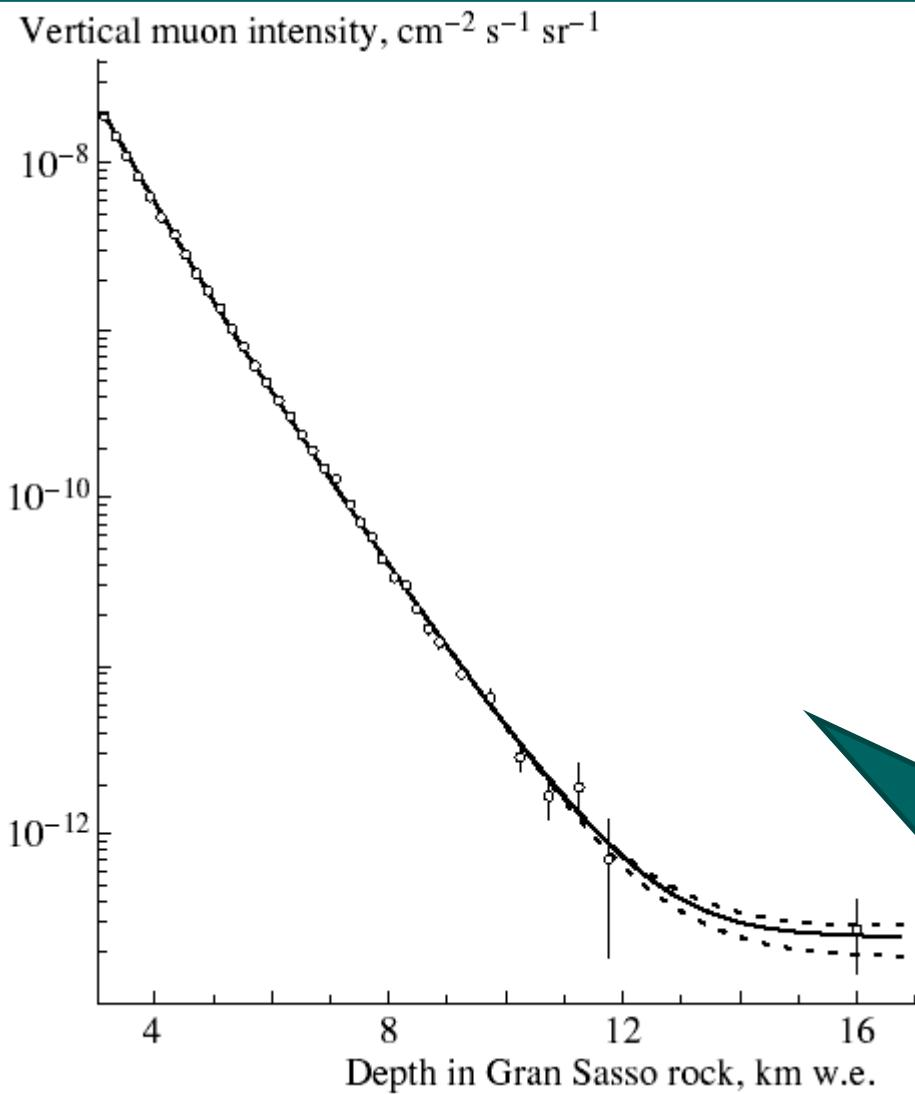
Depth–vertical muon intensity relation in Gran Sasso rock. The LVD data are presented together with the best fit (solid curve). Dashed curves show the calculated intensities for the maximal and minimal contributions from neutrino-induced muons (see text for details).
