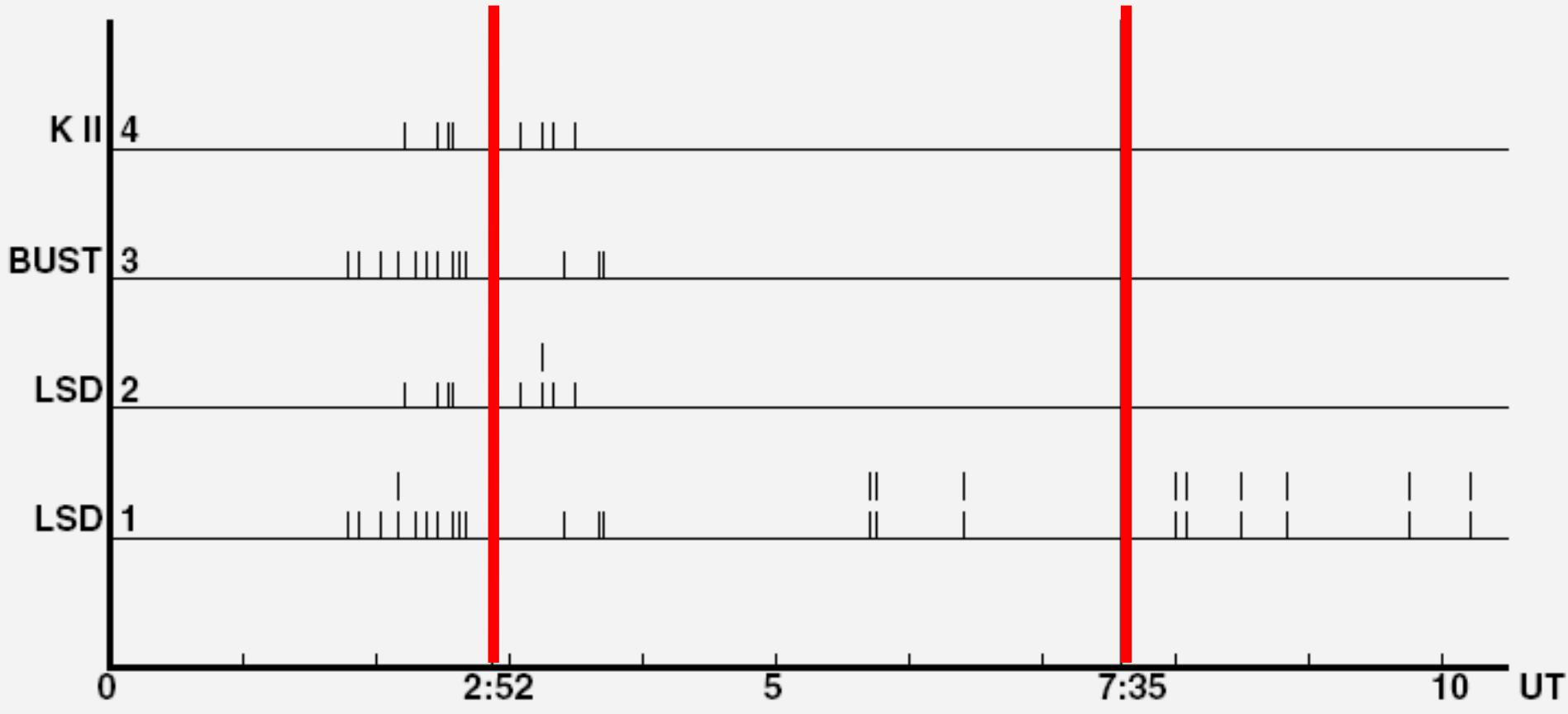
Timing diagram of the BUST pulses coincident with the LSD pulses within 1 s and similar coincidences for the K2 and LSD detectors as well as double pulses in LSD over the period from 0:00 to 10:00 UT on February 23, 1987.
