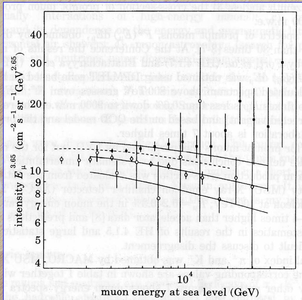
Vertical muon energy spectra at the sea level: diamonds: LVD data; circles: ASD data; bold boxes: MSU data; solid curves: LVD best fit ( $\gamma=2.75$ ) together with the error corridor of the parameters and absolute flux normalization; dashed curve: MACRO best fit
