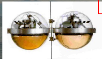
Quasar photodetector ( \varnothing=37\text{cm} )
